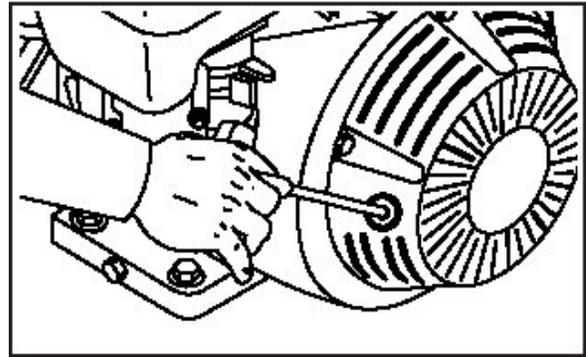
**STEP 10:** Pull the starter grip. If the engine fails to start after 2 pulls, squeeze the trigger gun to release pressure and repeat step. Return starter gently. After the engine warms up enough to run smoothly, move choke to run position and throttle to fast position.
