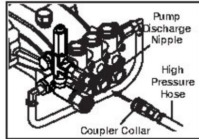
**STEP 3:** Connect the high pressure Hose to the pump discharge nipple. Push coupler collar forward until secure.
