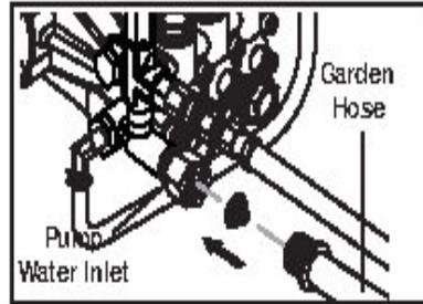
**STEP 5:** Check inlet filters, remove debris, then connect the garden hose to pump water inlet.
