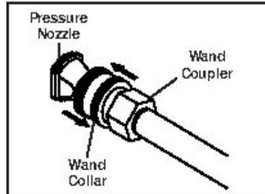
**STEP 2:** Release the coupler collar and push the nozzle until the collar clicks. Pull the nozzle to make sure it is sealed properly.
