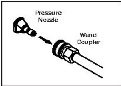
**STEP 1:** Pull the spring-loaded collar of the wand coupler back to insert your choice of pressure nozzle.
