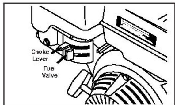
**STEP 8:** Move the choke lever to the "Choke" position (on a warm engine, leave the choke lever in the run position). Move the choke lever to the "Closed" position. To restart a warm engine, leave the choke lever in the "Open" position.
