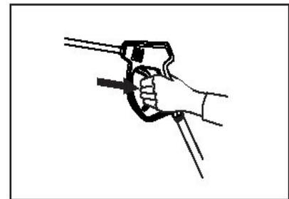
**STEP 6:** Trigger the spray gun to Eliminate trapped air then wait for a steady flow of water to emerge from the spray nozzle.
