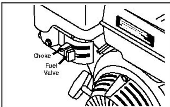
**STEP 7:** Rotate the fuel shut-off valve to the "On" position. Slide the fuel valve lever to the "On" position. When the engine is not in use, leave the fuel valve in the "Off" position.
