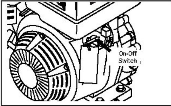
**STEP 9:** Turn the engine switch to "On" position. On Briggs engines, move the throttle lever to "Fast" position, shown on the engine as a rabbit.
